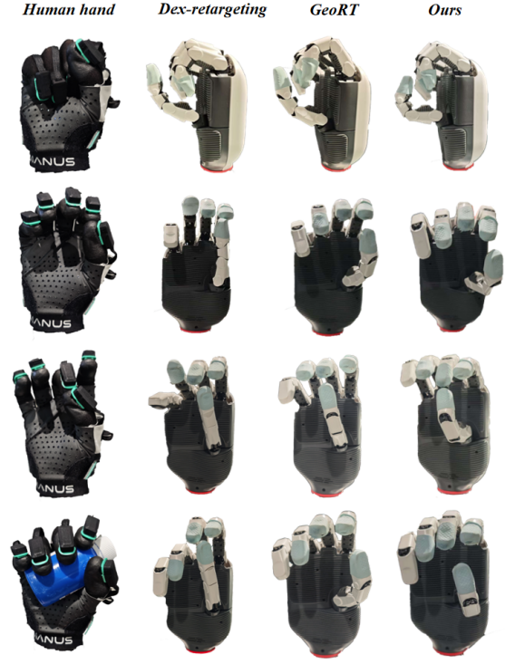
Fig. 4: Visualization of retargeting results for four representative gestures. We show the input human hand poses and the corresponding configurations generated by Dex-retargeting [35], GeoRT [24], and our method . Compared to other methods, our retargeting algorithm generates more accurate, smooth, and coordinated hand poses.
