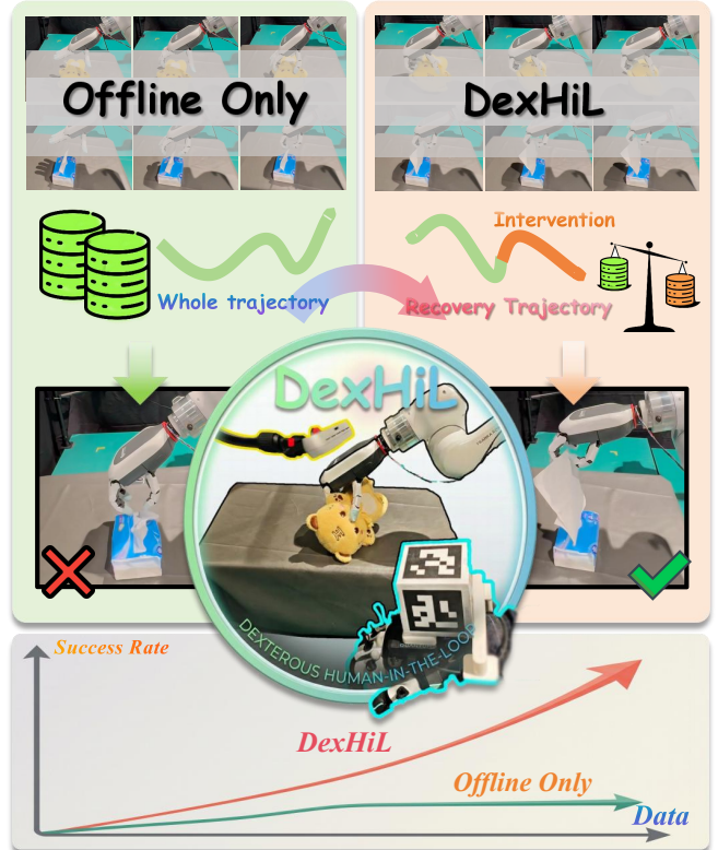
Fig. 1: While scaling offline data for VLA models yields slow accuracy gains and performance plateaus, DexHiL integrates offline training with online Human-in-the-Loop interventions. By strategically reweighting offline and corrective online data, our approach achieves high data efficiency and rapid accuracy growth.
